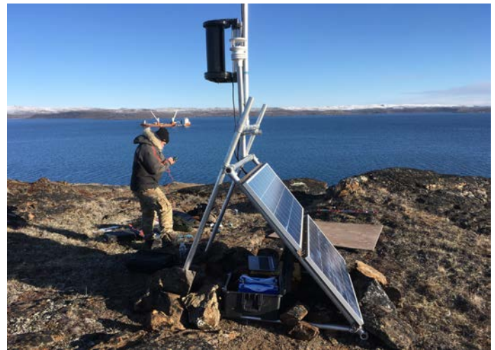
Figure 3. A remote/off-grid AIS unit used by the IMMP.
